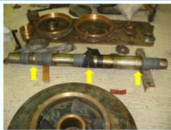
Shaft after rebuilding to frictions area with stainless steel electrode
