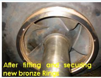
Impeller machining for fitting new Bronze Rings
