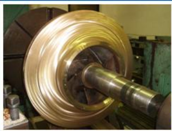
Impellers/Shaft on standard measurements during dynamic balancing
